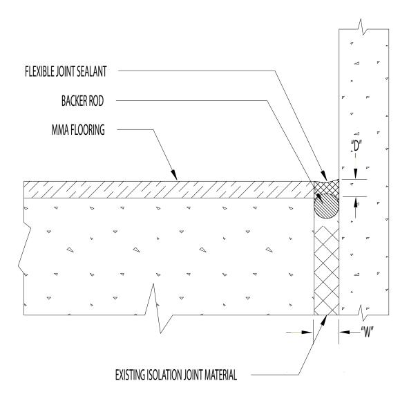
D = W /2 D = DEPTH OF BACKER ROD W = WIDTH OF JOINT
