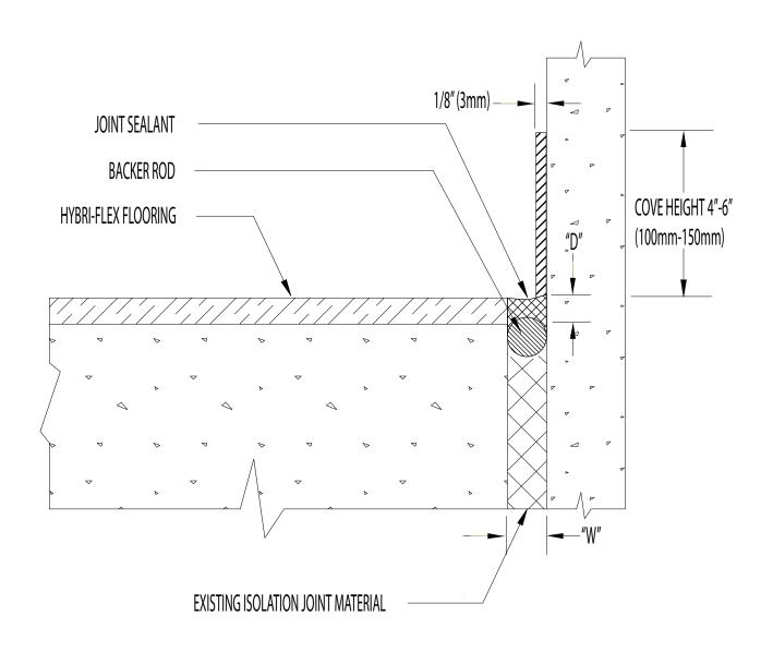
D = W /2 D = DEPTH OF BACKER ROD W = WIDTH OF JOINT
